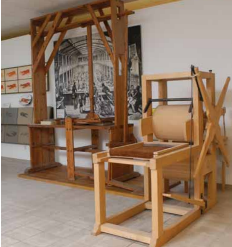
View of Room 4: Lithography The copperplate press and the bar press can be seen
